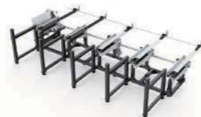
Semi automatic loading and unloading system
