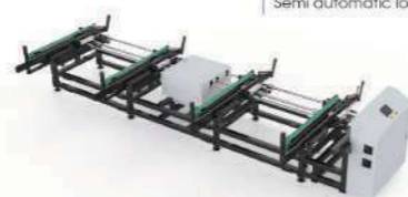
Semi automatic loading and unloading system
