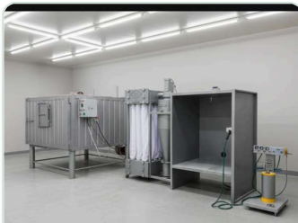
Complete Powder Coating Setup Integrated booth & recovery system
